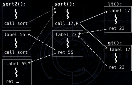
Figure 1: Example program fragment and an outline of its CFG and CFI instrumentation.
